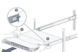
Loosen and remove the rail screws. Slightly pull out the middle latch as illustrated, and slide forwards to remove the inner rail from the chassis.
