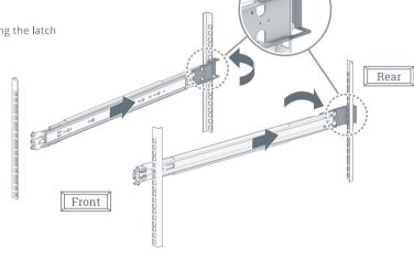
Adjust the length of the rail kit assembly, and insert the front end to the rack by slightly sliding the front latch outwards and inserting the brackets into the rack holes.
