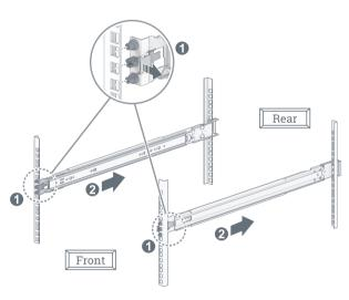
Pull the rear latch of the inner rail assembly, and slide forwards to remove the assembly from the rack.
