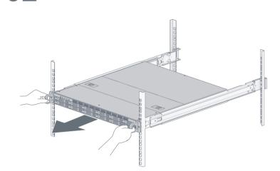
Slide outwards the rear latch of the inner rail to unlock the inner rail from the outer rail assembly. With the help of another person, carefully remove the chassis from the rack. (You may remove all drives first to reduce the weight of the chassis.)
