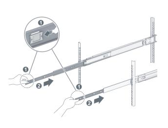
Push the front latch of the inner rail assembly, and slide backwards to remove the assembly from the rack.
