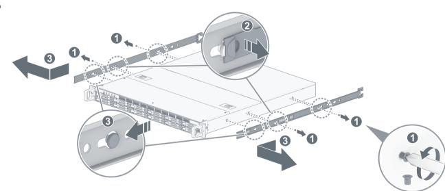
Insert the inner rail to the rail kit assembly by pulling outwards and holding its front latch.
