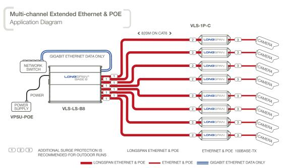
The diagram shows one of many possible configurations for a LONGSPAN Base 8 installation. In this example all channels are
