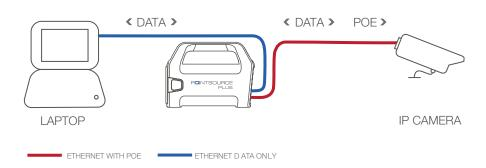
POINTSOURCE Plus delivers Ethernet and POE Plus to an IP camera for installation and set-up.
